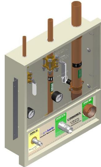
Shown above: Model PX-HCBU3OHW2A6VT Two valve+ One vent box with gauges 3/4" Oxygen valve & high flow oxygen (without check), 1/2" medical air, 1 1/2" oxygen vent
