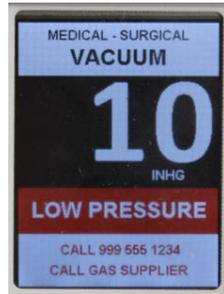
Shown in normal condition. Code specific gas colors, and gas name are displayed at the top in facilities language. Gas pressure and units of measure are displayed in the middle of the screen. Normal or Alarm condition is displayed in the bottom center. Rooms/area monitored alternates with user programmed emergency instructions at the bottom.
