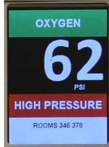
Shown in alarm condition displaying emergency instructions. Display blinks on and off when in alarm condition drawing attention and alternates displaying rooms/area monitored with user programmed emergency instructions.
