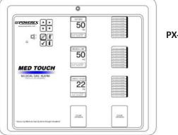
PX-T3IOAVF+++F = 3 Slot Combination Alarm Powerex labeled, set for ISO Color Code English/French gas set. Oxygen, Medical Air and Medical Vacuum, one Future Expansion (Blank) position at bottom, of 2nd slot 24 Dry Contact Signal Points w/ Latching Alarm Relays and one Future Expansion (Blank) position at bottom of 3rd slot. No Interface Communication Option.
