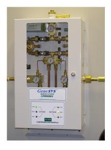
The control panel shall incorporate a set of LED's for each bank, green for "Bank in Use", amber for "Ready" and red for "Empty". Analog gauges are also provided so that line and both bank pressures may be observed.
