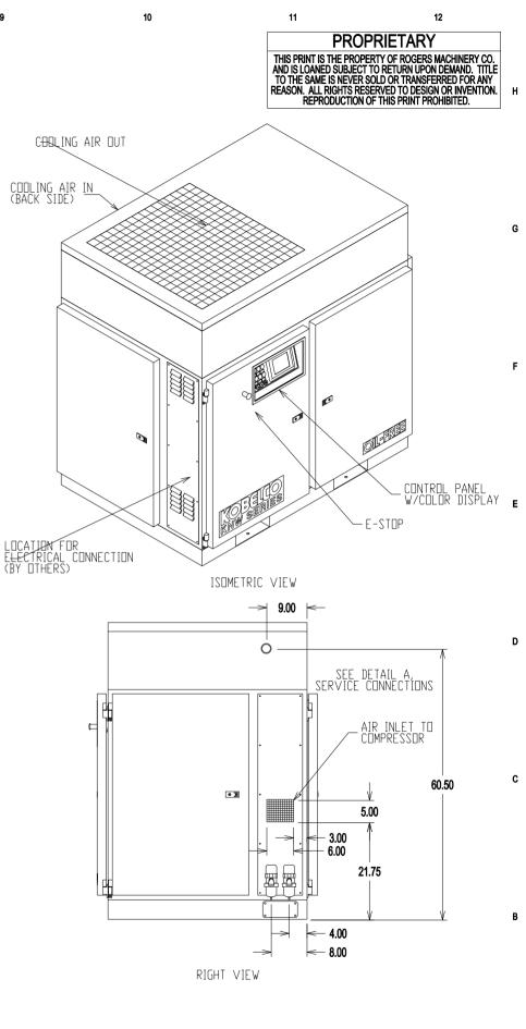
COMPRESSOR ASSEMBLY KOBELCO KNW SERIES AIR COMPRESSOR MODEL KNWA0, AIR-COOLED VYE-DELTA STARTER, STANDARD ASSEMBLY DRAWING NUMBER K00754A.0 SHEET 1 OF 1
