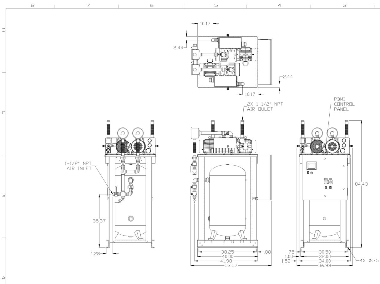
NDTE: A MINIMUM DF 24" CLEARANCE IS RECOMMENDED AROUND THE ENTIRE UNIT.
