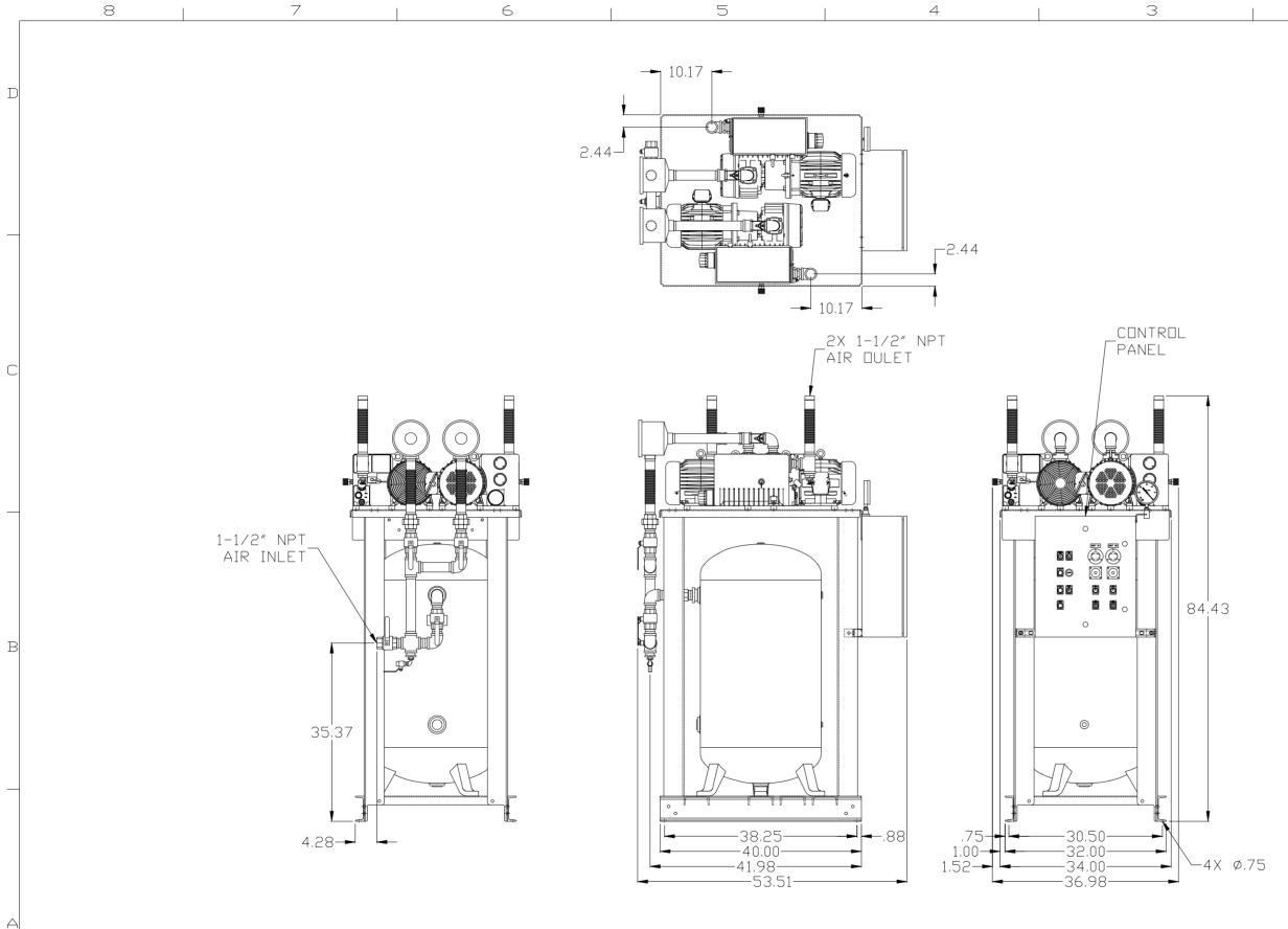
NDTE: A MINIMUM DF 24" CLEARANCE IS RECOMMENDED AROUND THE ENTIRE UNIT.
