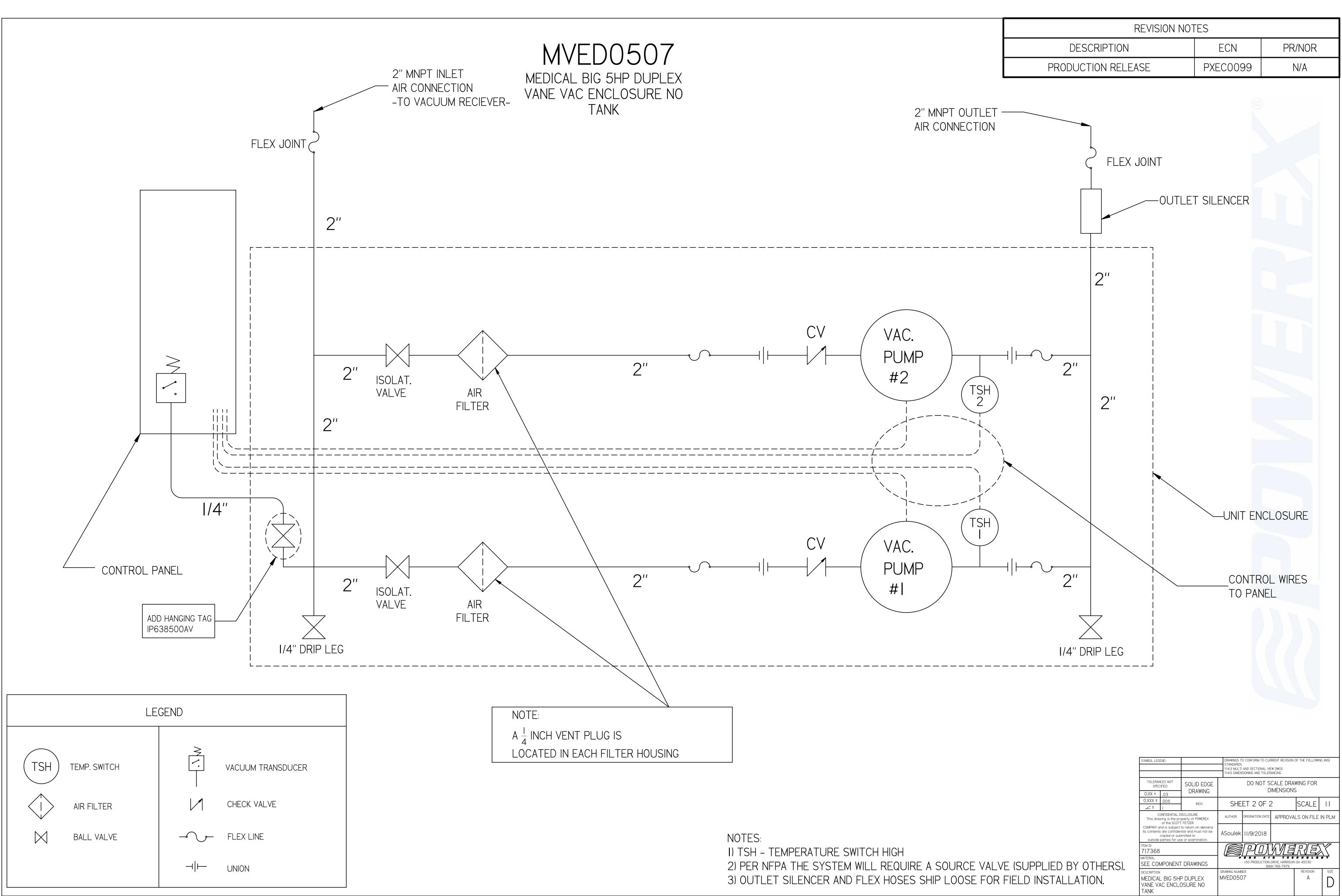
3) OUTLET SILENCER AND FLEX HOSES SHIP LOOSE FOR FIELD INSTALLATION.
