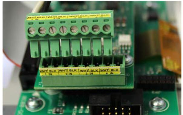
The sequence in which the transducers are connected to the board correspond with the order in which they will appear on the display. The #1 transducer will be displayed on top and the #4 transducer will be displayed on the bottom. There will be up to two display positions (high line pressure and low line pressure) for each transducer.
