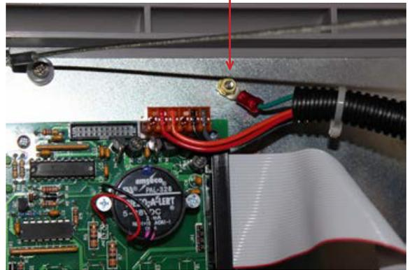
Attach the plug connector at the end of the wiring harness to the appropriate connector located at the top left corner of the button module circuit board. The plug should lock into place. The plug can only be inserted one way.
