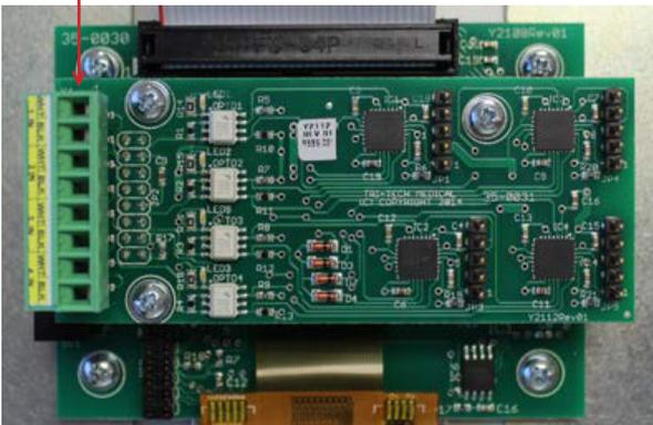
There are a total of 8 connection points – two connection points for each transducer sensor. The pairs are labeled 1 IN thru 4 IN on the circuit board. **The white wire from the transducer should be landed in the WHT position and the black wire from the transducer should be landed in the BLK position.** Note: only Powerex D and T series alarm transducers are compatible with the Med Touch alarm system.
