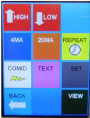
There are a few new Icon buttons that are unique for this module. The 4MA icon is used to set the numeric value that a 4mA signal will represent based on the units you will be using i.e. 100 gallons. The 20MA icon is used to set the numeric value that a 20mA signal will represent i.e. 2000 gallons. These values will represent the span of the 4-20mA device.
