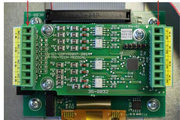
There are a total of 16 connection points – two connection points for each remote signal. The pairs are labeled 1 IN thru 8 IN on the circuit board. **The NC (normally closed) labeled terminal of each pair is where the signal wire should be landed. The C (common) labeled terminal of each pair is where the common wire should be landed.** **Note: it is required that polarity be maintained between the switch being monitored and the master alarm.**
