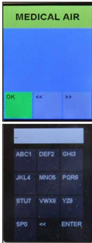
Below are examples of a completed Text display screen and how it appears as displayed as part of the gas or transducer master display. When an alarm occurs the emergency instructions will appear alternately with the normal information label.
