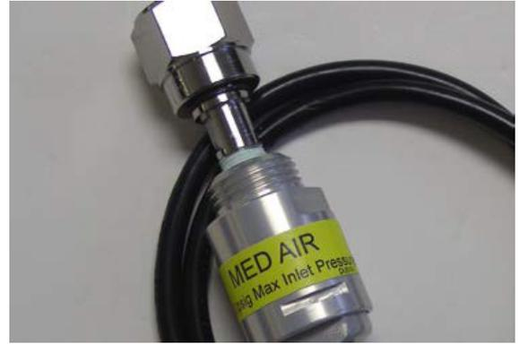
A panel mount feature has been provided to allow mounting of the transducer using standard 1/2" conduit connections and 4"x 4"x 2 1/8" junction boxes. Note: The DISS nut & nipple will need to be removed to allow installation of the conduit nut and then re-installed using oxygen safe Teflon tape.
