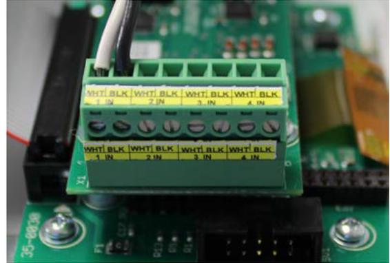
The connector terminal may be un-plugged from the circuit board to simplify installation of the remote signal wires.
