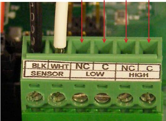
The other four connection slots are for optional remote monitoring of the low and high line pressure alarms on a master alarm, building management system, or other device.
