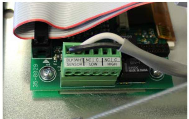
The other four connection slots are for optional remote monitoring of the low and high line pressure alarms on a master alarm, building management system, or other device.
