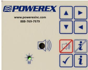
The Push Button module includes a power on indicator, quick view information buttons, the silence button and an audible alarm.
