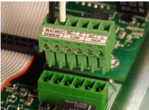
The transducer plug may be removed from the gas module to make it easier to install the wires.
