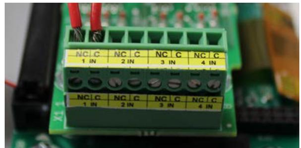
The connector terminal may be un-plugged from the circuit board to simplify installation of the remote signal wires.
