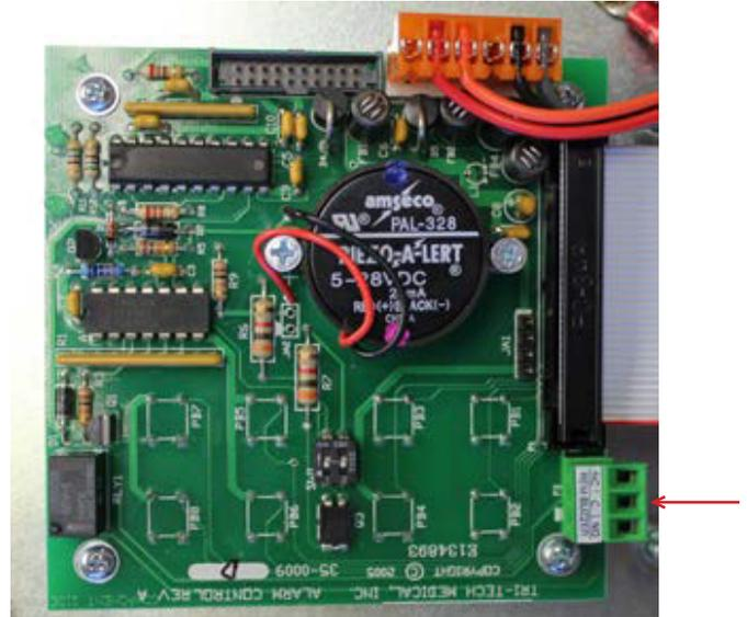
Normally Open (NO), Normally Closed (NC) and Common (C) connections are provided.
