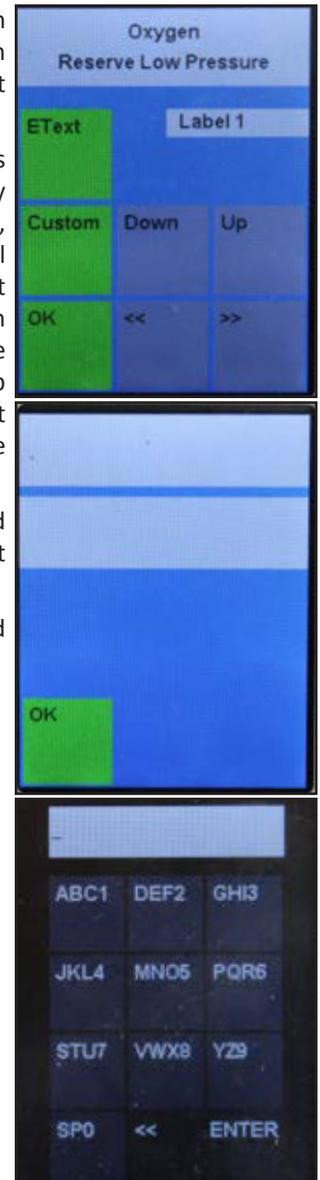
Below are examples of a completed Text display screen and how it appears as displayed as part of the master board display. When an alarm occurs the E Text emergency instructions will appear alternately with the normal alarm signal label.
