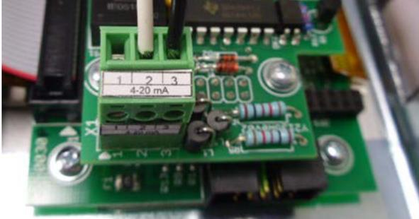
For 4-20mA transmitters with loop power supplied by the Alarm Circuit Board (35-0037)
