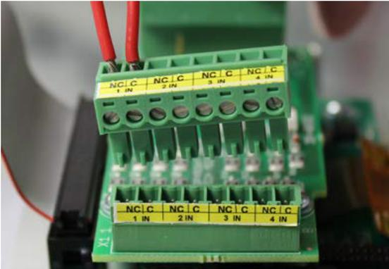
Land the corresponding signal on the NC (normally closed) & common wires on the C (common) terminal of each pair of terminal connectors. It is imperative that the signal wires are landed in the NC position and that the common wires are landed in the C position.
