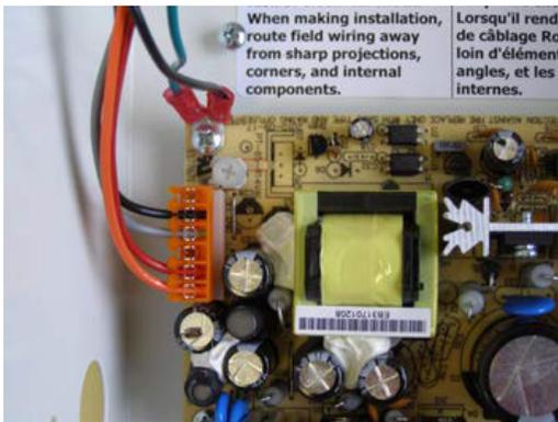
This is how the power supply should look when the wiring is completed.
