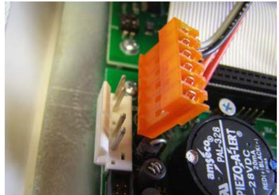
This is how the wiring harness plug connector should look when properly installed on the back of the button module board.
