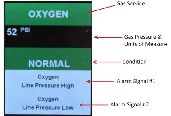
Emergency instructions may also be input (by the user) for each of the signal points. The normal display will appear and react just like a conventional remote signal master dry contact display (shown on the left side of this page), but a touch of the display will change the display (for 30 seconds) to look and react similar to an area alarm gas display (photo at right). The advantages of using transducers over pressure switches are;
