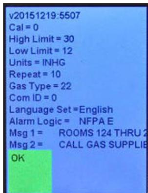
programmed for the board. The Com ID number is the communication ID number which has been programmed for the board. The Language Set is an abbreviation for the label set which has been programmed for the board. The Alarm Logic is the latching or non-latching software which has been programmed for the board. MSG 1 are the rooms or area(s) covered by the alarm. MSG 2 are the emergency instructions programmed for the board.
