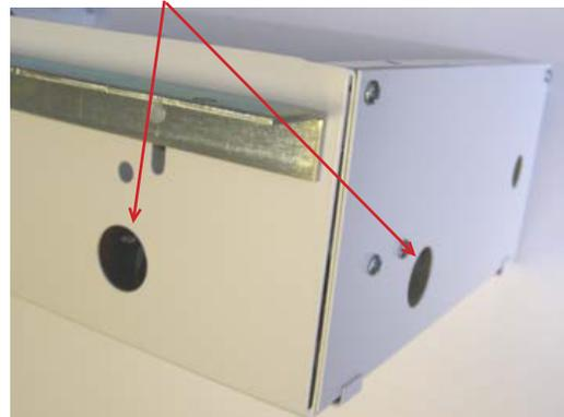
Route wires through the power supply conduit installed in the bottom and left side of the rough-in box. Connect the 120 or 240 VAC facility emergency power source electrical wiring to the terminal strip provided on the lower left side of the box. (N = neutral, L = Line (hot), FG = field ground).
