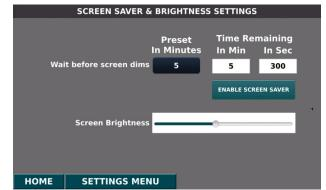
The Powerex FirstCall<sup>™</sup> Manifold is factory-set with a 5 minute screen saver. The screen goes dark after 5 minutes, but reactivates if there is an alarm or if the screen is touched.
