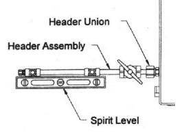
Remove the U-bolt assemblies from the header mounting brackets. Position the brackets so that the top of the bracket is aligned with the bottom of the headers and is centered between the cylinder connections. The end bracket should be placed as close to the last cylinder as possible to provide the most support and stability.
