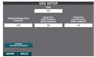
The Gas Setup screen displays the default UOM, default changeover pressure, default final line high pressure alarm setpoint, default final line low pressure setpoint, and default emergency reserve low pressure setpoint.
