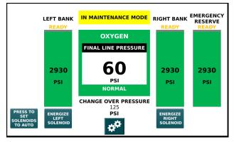
Pressing these buttons will toggle the "IN USE" status to that bank. To switch over to the right bank, press the "ENERGIZE RIGHT SOLENOID" button. To switch to the left bank, press the "ENERGIZE LEFT SOLENOID" button.
