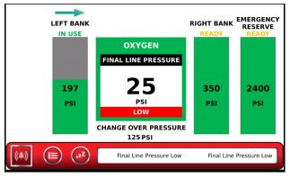
Close the bleed valve on the left final line regulator and SLOWLY reopen the cylinders on the left bank. The left bank pressure gauge and graphical display should return to full pressure. The left bank will now show "READY" above the cylinder graphic. The Changeover to Secondary Supply alarm will stop.
