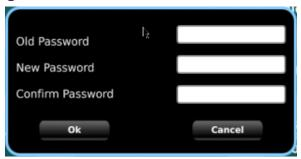
To change the password, press the "Change Password" button, enter the old password, enter the desired new password, and confirm the desired new password.
