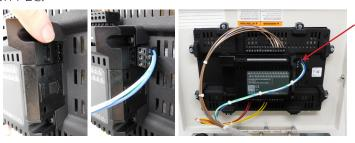
(For panels with 39+ digital inputs and/or 5+ gas inputs) Plug I/O module expansion adapter cord into appropriate port.
