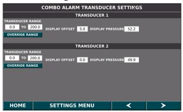
The Powerex FirstCall™ Area and Combo Alarm Systems come with the ability to adjust the displayed value of the pressure, as well as override the standard pressure range of the installed transducer.
