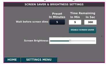
The Powerex FirstCall™ Alarm System is factory-set with a 5 minute screen saver. The screen saver dims the panel to 10% after 5 minutes. This time limit can be changed. The boxes to the right show the time remaining until the screen saver is enabled.
