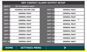
Standard dry contact output is on terminal block "O0" for General Fault.
