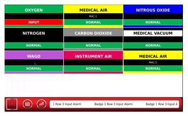
To see the specific alarm, press the gas badge that's in alarm to view the list of alarm conditions. The specific alarm will be highlighted in red.
