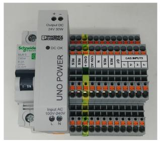
Ground wire – Strip ½" of insulation and connect the ground wire to the appropriate terminal block (GND).
