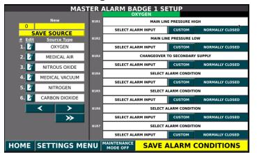
The Master Alarm Settings screen is where the source equipment gas is identified and alarm signal inputs are assigned. Up to 12 Source Badges are available, with up to 7 digital input signals available for each source badge. Please note that Powerex FirstCall™ Master Alarm panels are available in either 23, 39, and 55 digital inputs.
