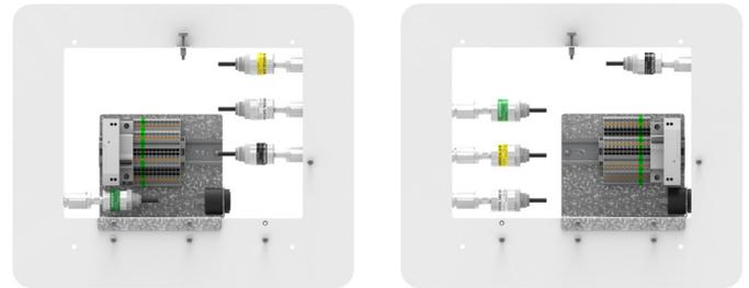
Position the cover plate and electronics bracket assembly on the wall with the bracket assembly inserted into the existing rough-in. The cover plate must cover the rough-in and any gap in the drywall around it, and the electronics bracket must be fully recessed into the rough-in without contacting anything on the sides or back of the rough-in.
