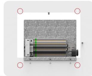
Drill holes in all 4 locations and install the insert portion of the drywall anchors – drill bit size and anchor inserts should all be done per the drywall anchor manufacturer specifications. Powerex does not provide fasteners or drywall anchors as part of Retrofit kits.
