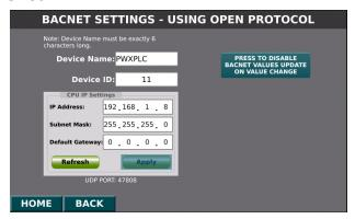
Enter desired device name – must be exactly 6 characters. Default name is always PWXPLC.
