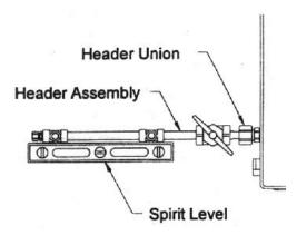
Remove the U-bolt assemblies from the header mounting brackets. Position the brackets so that the top of the bracket is aligned with the bottom of the headers and is centered between the cylinder connections. The end bracket should be placed as close to the last cylinder as possible to provide the most support and stability.
