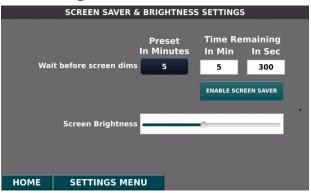
The Powerex FirstCall™ Manifold is factory-set with a 5 minute screen saver. The screen goes dark after 5 minutes, but reactivates if there is an alarm or if the screen is touched.
