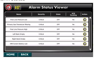
The Alarm Status screen shows a list of all possible alarm conditions for the maximum number of gases and input signals available in the Powerex FirstCall  $^{\text{TM}}$  Alarm System.
