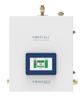
without fluctuation in line delivery pressure. Each bank goes through two stages of pressure regulation, beginning with the dome-loaded bank regulators and then the piston-style final line regulators. After the depleted cylinders are replaced, the manifold automatically designates that bank as the reserve supply, with no manual resetting of valves or levers required.
