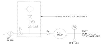
The Powerex control will close the isolation solenoid and open the purge solenoid when Auto-purge is active. This will allow fresh clean air to be drawing through the small filter assembly. The manual control valve between the air filter and purge control solenoid should be opened so that the vacuum level on the gauge is between 19 and 20 inches Hg.
