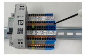
Install the sensor wires into the appropriate terminal block. There are enough terminal blocks for up to 8
