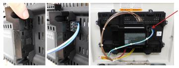
(For panels with 39+ digital inputs and/or 5+ gas inputs) Plug I/O module expansion adapter cord into appropriate port.
