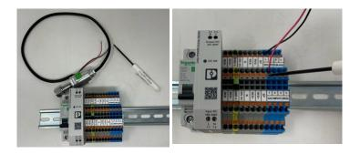
It is important that the sensors are wired to the correct terminal block. Per NFPA 99, an alarm will sound for cross-connected sensors.
