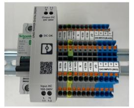
Ground wire – Strip  $\frac{1}{2}$ " of insulation and connect the ground wire to the appropriate terminal block (GND).
