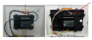
Plug power cord from power supply into power slot on PLC.
