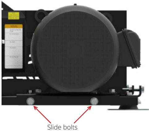
3. Loosen the tensioning bolt until enough slack is available to remove the old belts.
