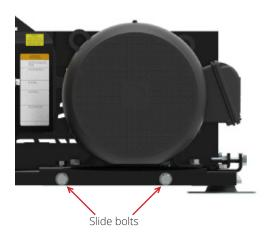
3. Loosen the tensioning bolt until enough slack is available to remove the old belts.
