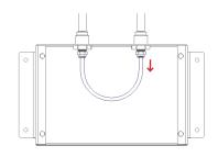
6. Disconnect the gas outlet tube from the fitting inside the back box.
