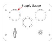
15. A Supply Pressure Gauge (or Inlet Pressure Gauge) is provided to allow monitoring of the pressure being supplied to the gas control panel. The pressure shown on this gauge will match the pressure shown at the zone valve box provided the Supply Valve on the gas control panel is ON or open.
