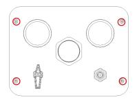
12. Attach the front panel to the back box (using the 4 long screws provided). Be careful not to pinch or damage tubing. The tubing connectors swivel to ease installation. Remove shipping cap.
