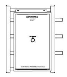
13. The Gas Control panel should now be ready for testing and use. To restore gas service to the panel, locate and open the zone valve providing gas to the gas control panel.
