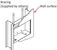
1. Provide rigid mounting that will support the gas control panel back box on the top and bottom. (Rigid mounting materials are not included with the panel). Refer to the building plans to determine location of the panel. Mount back box so it will be flush or just below the finished wall surface. Remove dust cover from back box only when the finished wall surface is complete and you are ready to install the front panel. Adjustable flange
