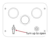
14. Use the Supply Valve on the gas control panel to control gas flow to the panel and equipment connected downstream of the panel.
