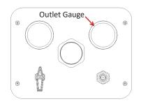
17. The Outlet Pressure Gauge displays the delivery or outlet pressure as controlled by the regulator.
