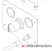
18. The Gas Outlet allows connection of DISS Gas hose assemblies. The outlet connection provides a demand check valve which automatically stops the flow of gas when the hose is disconnected. The Gas Control Panel is now ready for use!
